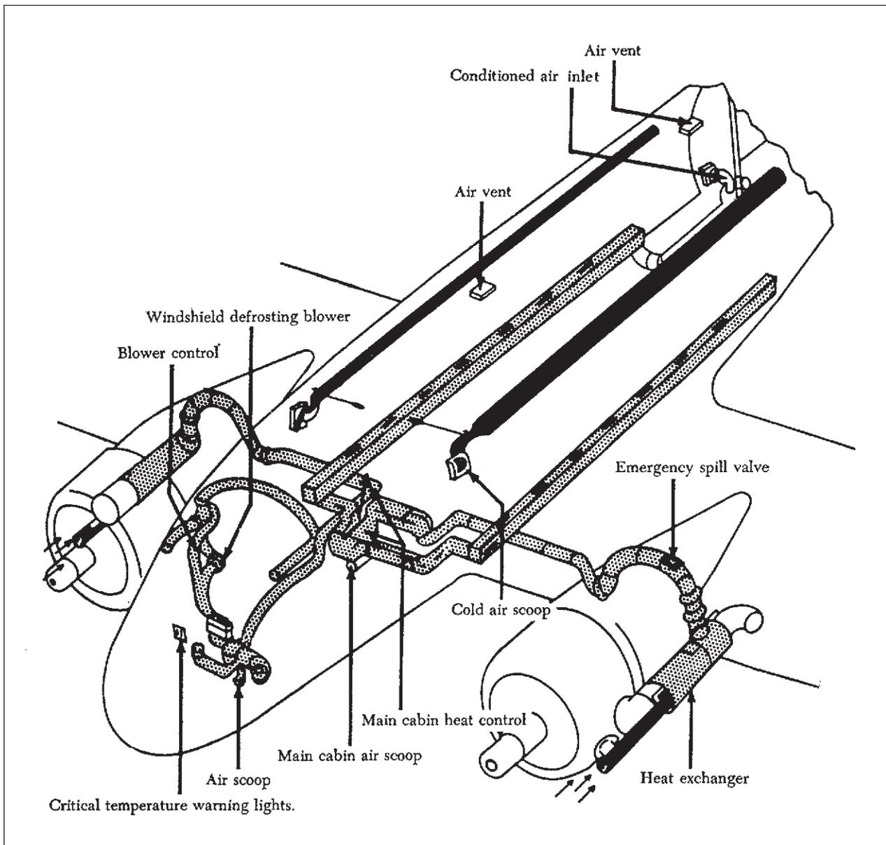
**Figure 1-27b Engine exhaust heater system.**
