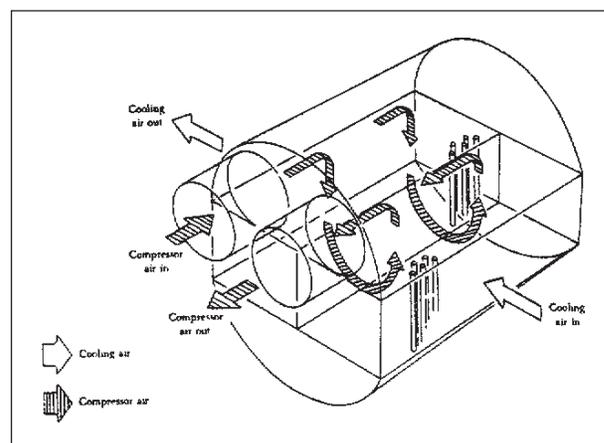
Figure 1-27a Schematic of primary heat exchanger.
