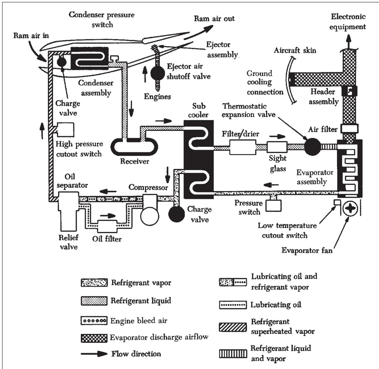
Figure 1-24 Vapor cycle system flow schematic.
