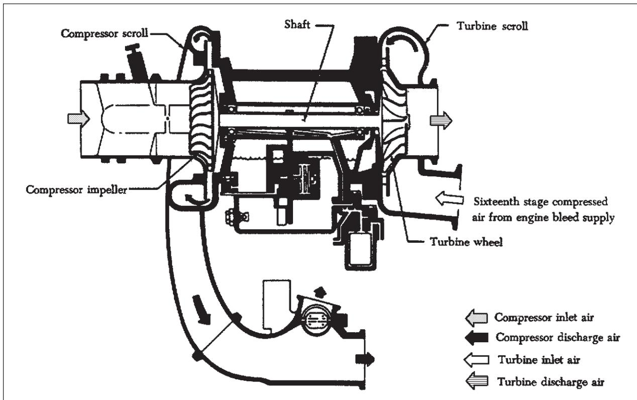
Figure 1-26 Schematic of air turbine centrifugal compressor.
