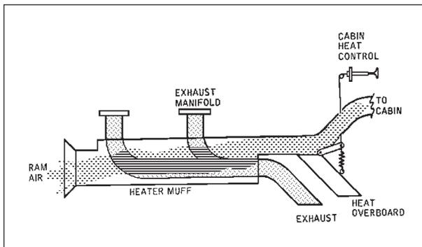
**Figure 1-28b** Exhaust heating system for a light airplane.
