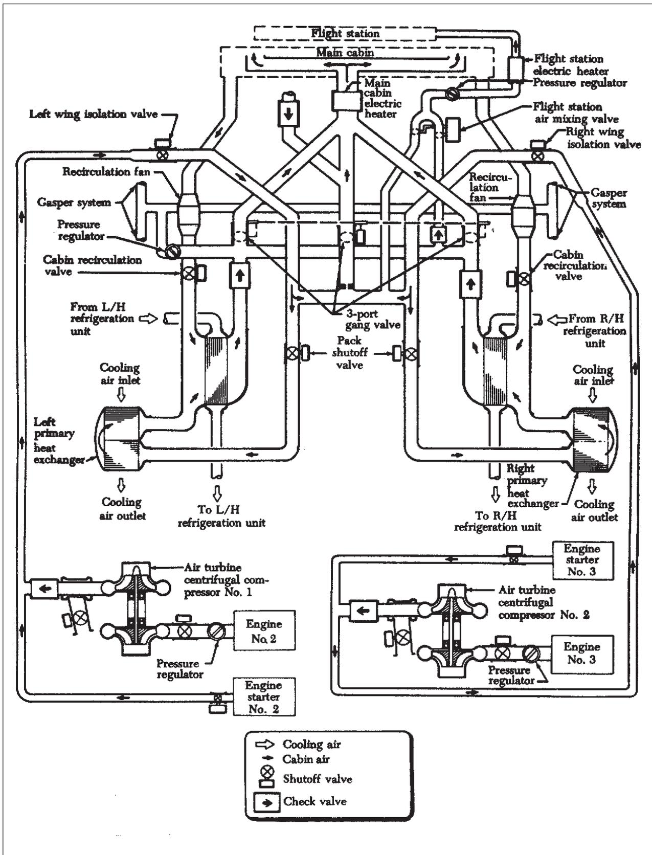
Figure 1-25 Schematic of vapor cycle air conditioning system on Boeing 707 and 720 airplanes.
